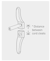
Mark the hole positions and drill as required.
